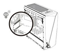
Remove the baffle marked in the picture, make sure the Graphic card aims at the motherboard slot and then fix Graphic card and case with No.1 screw.
