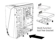
Multi-function tool free bracket support both SSD and HDD, put the SSD or HDD in the bracket to install
